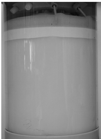
Figure 4. Annular chromatograph with two different separation media. At the bottom is the size-exclusion gel, above the ion-exchange resin and on top glass beads.
